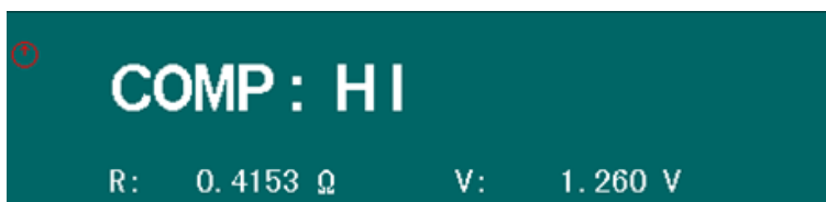
Figure 3.18: Compare Test - Above Limits
