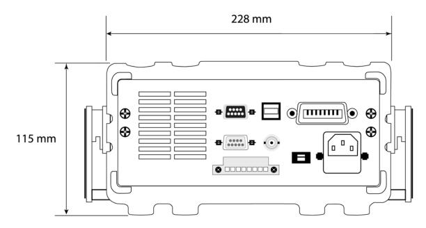
Figure 4 - Rear View (Half-rack models)
