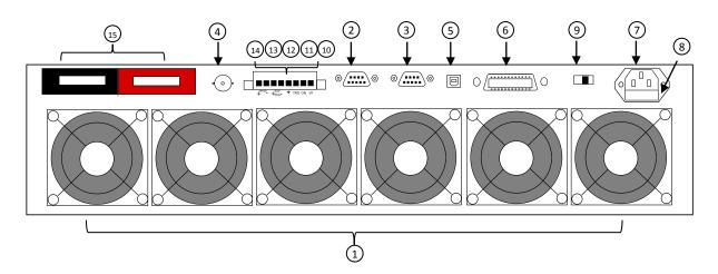
Figure 10 - Rear Panel (Full-rack models)
