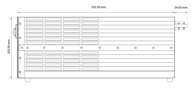
Figure 3 Front and Side View (Full-rack 6U models)
