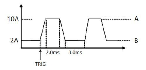
Figure 20 - Continuous Transient Operation Current Waveform
