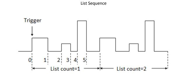
Figure 23 - List Mode Current Waveform
