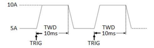
Figure 21 - Pulse Transient Operation
