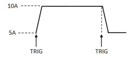
Figure 22 - Toggle Transient Operation
