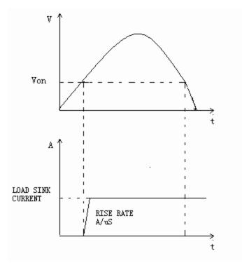
Figure 16 - Von Latch OFF The Load's Operating Range with Von Latch set to OFF
