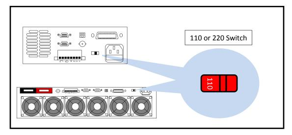
Figure 12 - Line Voltage Switch Location
