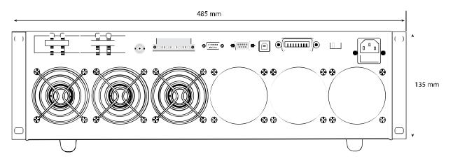
Figure 5 - Rear View (Full-rack 3U models)
