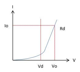
Figure 17 - CR LED IV Characteristics Curve
