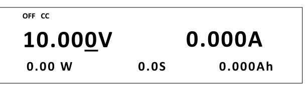
8. To start the battery test, press (Trig) once. The input will automatically be enabled (ON) with the On/Off button's backlight lit. The timer on the display will run continuously and Ah measurement will update through time. The test will continue to run until one of the three stop conditions is met.
