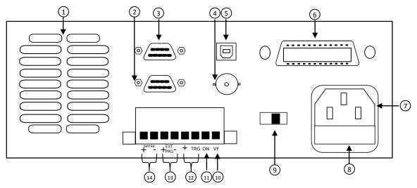
Figure 9 - Rear Panel (Half-rack models)
