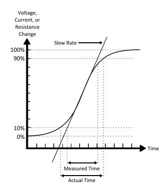
Figure 14 - Slew Rate Measurement
