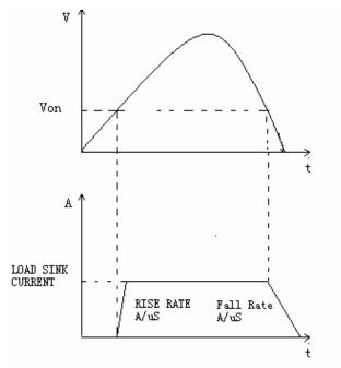
Figure 15 - The Load's Operating Range with Von Latch set to ON
