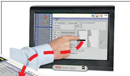
With Virtual Network Computing software, you remote control your DAS 800 from a computer or a tablet.
