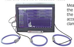
Measurements are done with the voltage input (direct) of the universal board and accessories clamps (standard clamps or flexible clamps)
