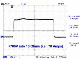
The AVOZ-D models are high-voltage, high-current pulsers that feature five, ten, or twenty identical outputs. These outputs can either be combined to drive a single low-impedance (2.5, 5 or 10 Ohm) load, or can be used separately to drive multiple 50 Ohm loads simultaneously. This unique flexibility makes the AVOZ-D series ideal for testing high-current laser diode arrays, as well as testing multiple identical lower-current devices (for instance, production testing of attenuators).
