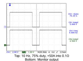
The AV-109E and AV-109F series of pulsed constant current generators are designed for driving laser diodes and other low impedance loads with constant current pulses as high as 100 Amperes, pulse widths from 10 us to 1 second, and average output powers of up to 200 Watts. All models will operate for load voltages in the range of 0 to 5V, making them suitable for most single-diode loads.
