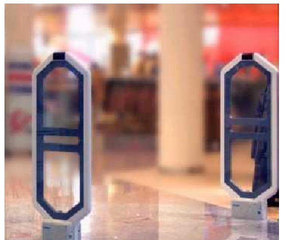
Magneto acoustic gate used for product surveillance
