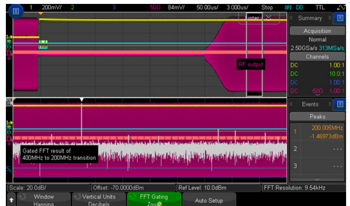
Figure 21d. RF signal settled down at 200 MHz as indicated in the search list.
