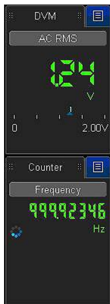
Figure 26. DVM and counter takes advantage of separate signal paths to provide measurements without a trigger, while still using the scope probes.
